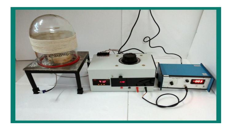
Applications: To test the IV characteristics with respect to temperature (Max Room temp—600 ° C) and sensitivity performance of compound material (in the form of thin film or pallet) at different gases.
